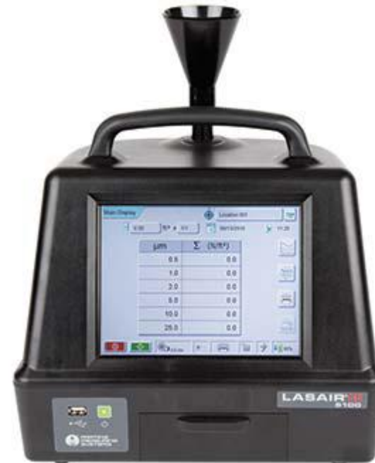
Particle counter Lasair III R For classification CR
