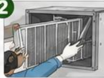
Pembersihan / penggantian pre-filter & medium filter
