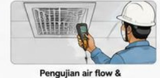
Pengujian air flow & air change rate (ACH)
