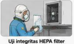
Uji integritas HEPA filter (PAO/DOP test)
