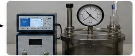
Uji kebocoran (He leak test)
