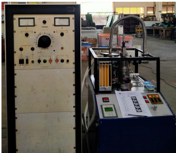
Gambar Alat DC Sputtering
