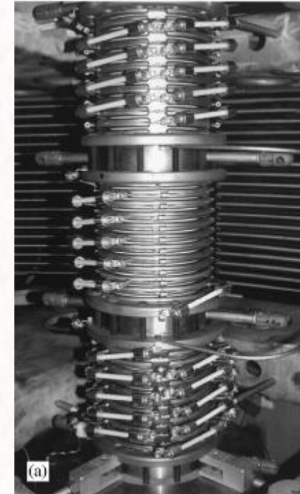
Tabung Pemercepat High gradient: (a) three short-tubes (old standard tubes) in a 1 MV module in the present 20UR tandem accelerator at JAERI-Tokai and (b) Two long tubes (so called compressed geometry tubes) for the replacement
