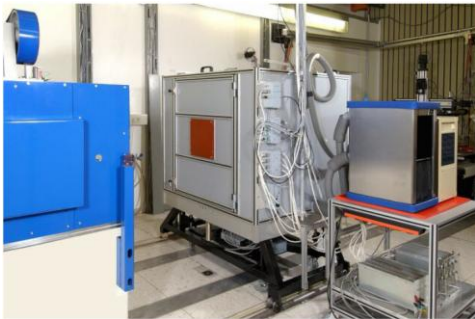
Figure 1. The PTB water calorimeter (centre of the picture) in front of the ^{60}\text{Co} radiation facility (left side). Shown is the calorimeter's outer container with the radiation entrance area (dark square). The coolers for maintaining the operating temperature of 4^\circ\text{C} and some of the associated electronics can be seen on the right side of the picture.
