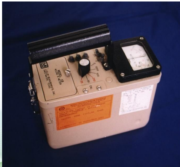
Gamma Radiation Exposure Micro R Meter Model 19 with NaI(Tl) Detector
