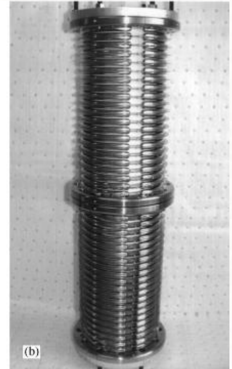
Tabung Pemercepat High gradient: (a) three short-tubes (old standard tubes) in a 1 MV module in the present 20UR tandem accelerator at JAERI-Tokai and (b) Two long tubes (so called compressed geometry tubes) for the replacement
