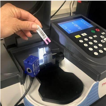
Spectrophotometer read the absorbance
