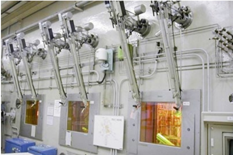
Concrete Cells for Highly Radioactive Material (Analysis and Research Center)
