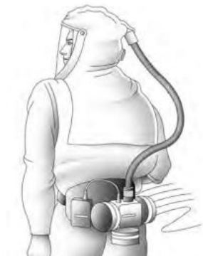
Hood Powered Air-Purifying Respirator (PAPR) APF= 25
