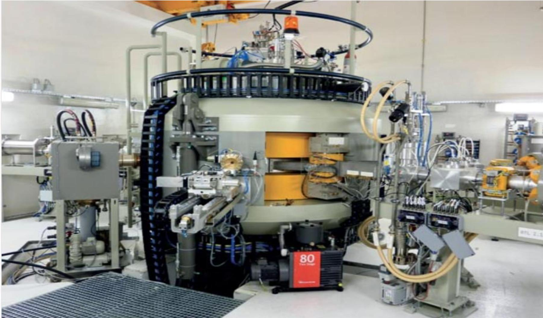
Fig. 2. The power-efficient Cyclone-30 isotope-producing cyclotron, 2.7 m in diameter and 2.8 m high.
