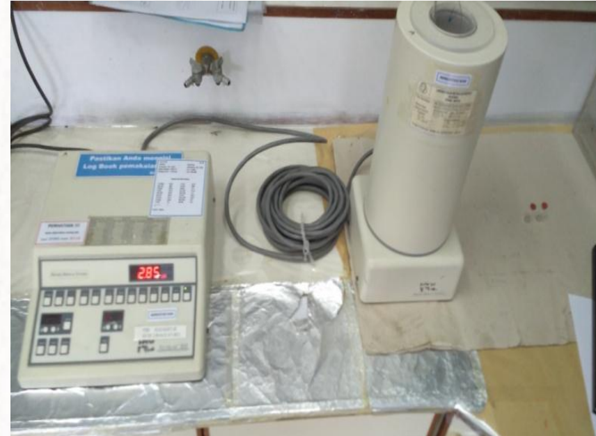
Dose calibrator (Gamma Ionization Chamber)
