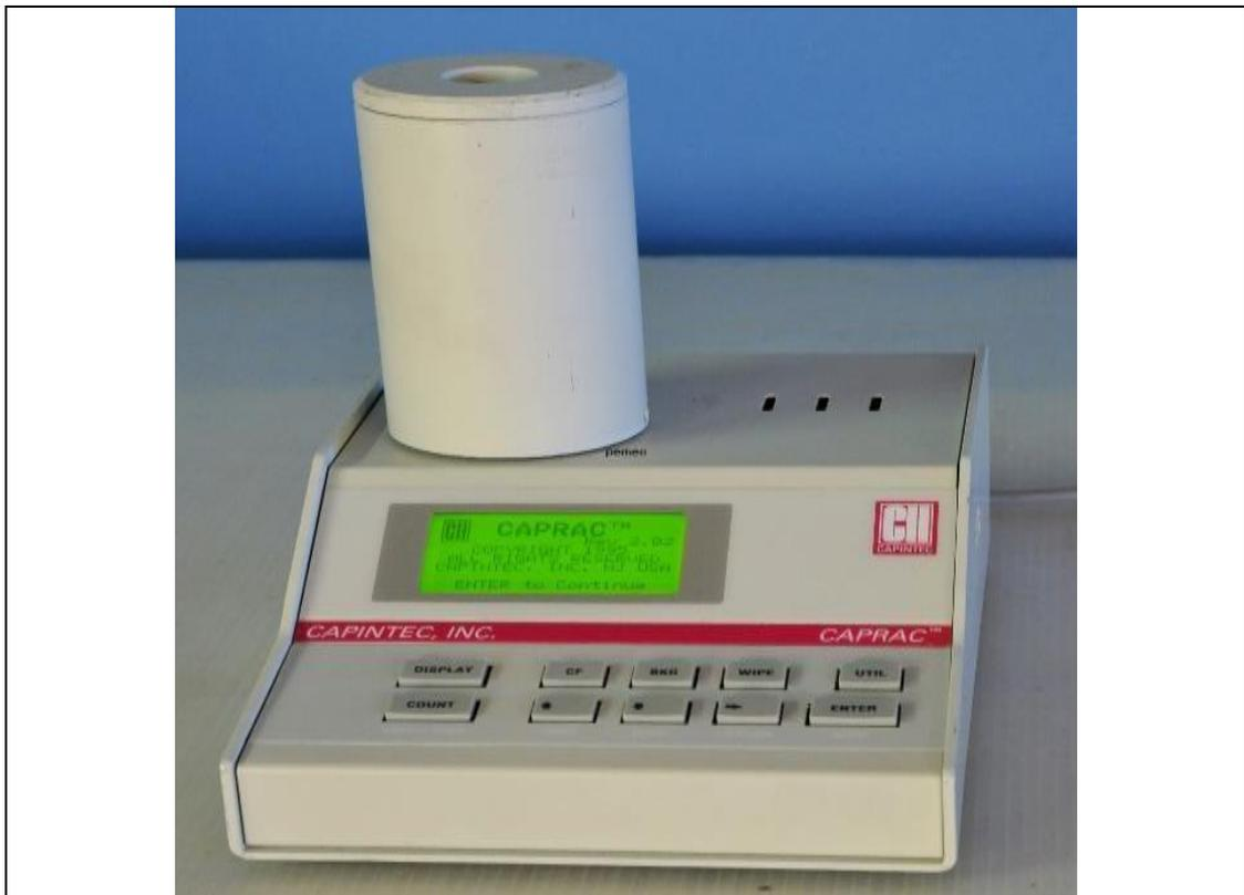
**Gambar 21.** Gamma Ionization Chamber (GIC)/ Dose Calibrator
