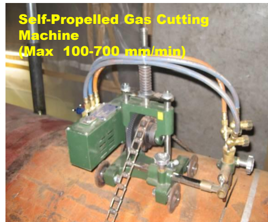
Cutting of feedwater heater
