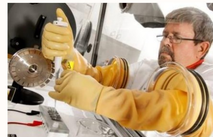
Loading solution onto Re filament
