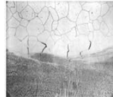
8.12 Hot cracking in a weld joint Hot cracking in a weld joint (chromium-nickel steel)
