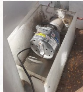
Staplex – HVAS (High Volume Air Sampler)
